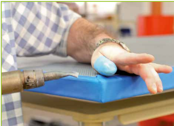
Down to the last detail: welds in BSW Martial Arts Mats are made meticulously by hand to warrant a precise fit, high strength and complete sealing.
