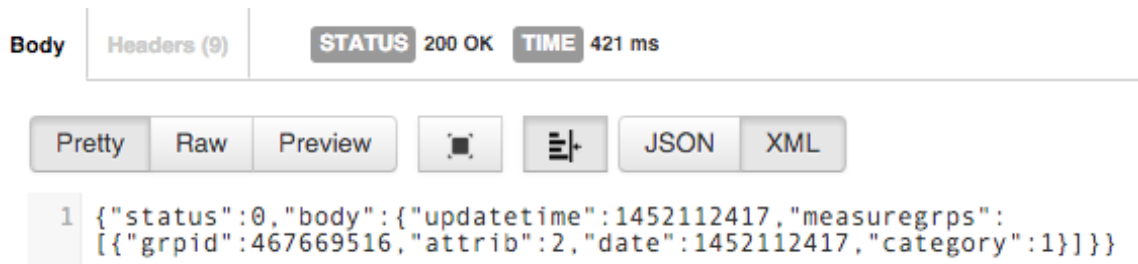
Figure 5: The Withings server responding to the HTTP request containing a falsified heart rate measurement. “Status: 0” indicates the server accepted the data. Other information present include the time at which the server accepted the request and the time associated with the heart rate measurement.
